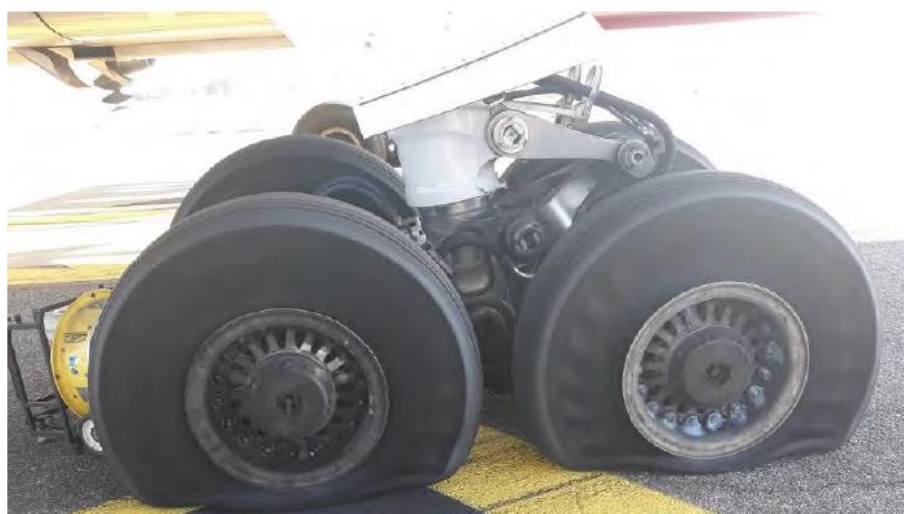
Picture 10: deflated left landing gear tires.
