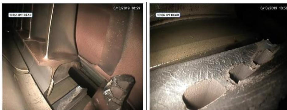
Picture 12: fracture surfaces of the IPT blades found broken.
