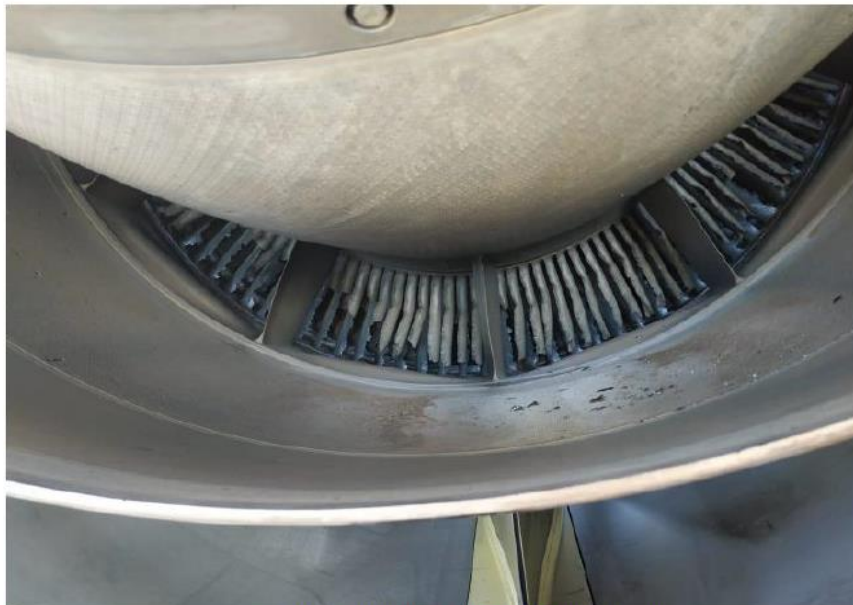
Picture 3: external evidence of left engine damage.
